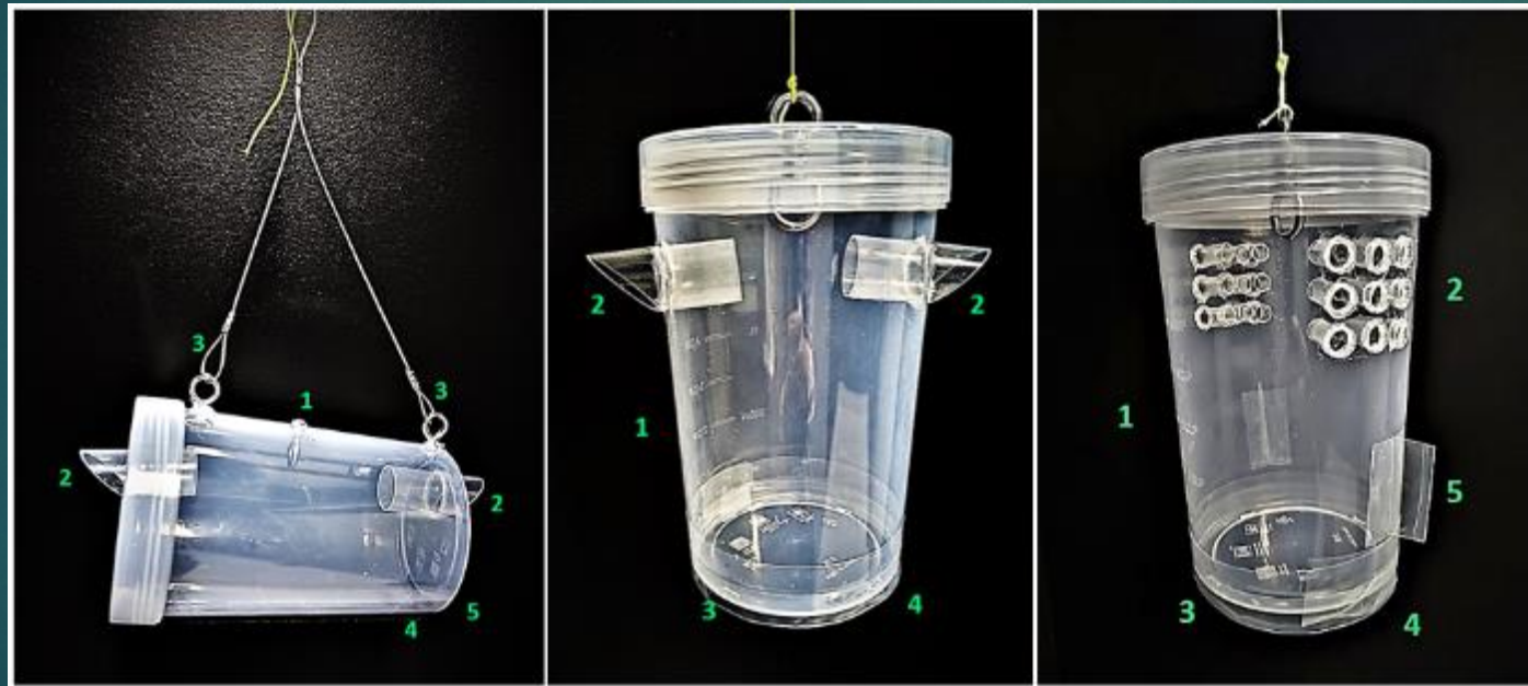
Enhanced Steiner trap (left), Paton trap version 1 (middle), Paton trap version 2 (right), showing new elements to reduce water entry.
